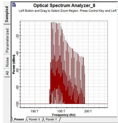
Figure 8: Input Spectrum for 32 Channels & 20 dbm Input Power
