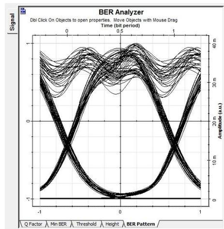
Figure 3: Eye Diagram for 32 Channels & 20dbm Input Power
