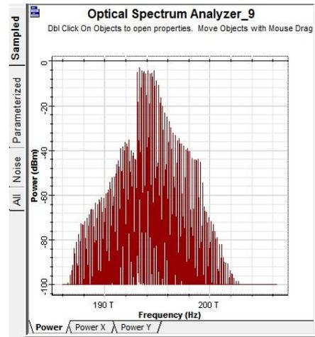
Figure 9: Output Spectrum for 32 Channels & 20 dbm Input Power
