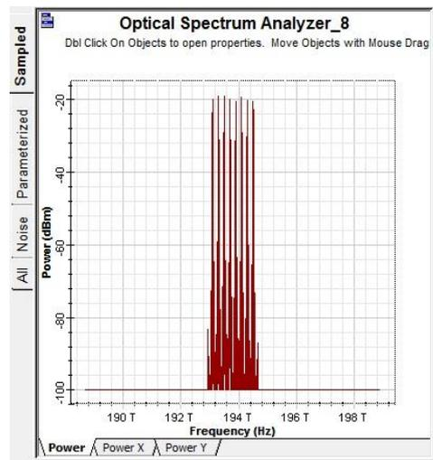
Figure 4: Input Spectrum for 8 Channels & 5 dbm Input Power
