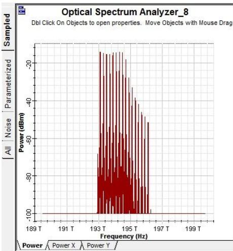
Figure 6: Input Spectrum for 16 Channels & 10 dbm Input Power
