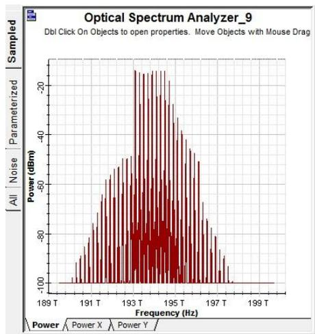
Figure 7: Output Spectrum for 16 Channels & 10 dbm Input Power
