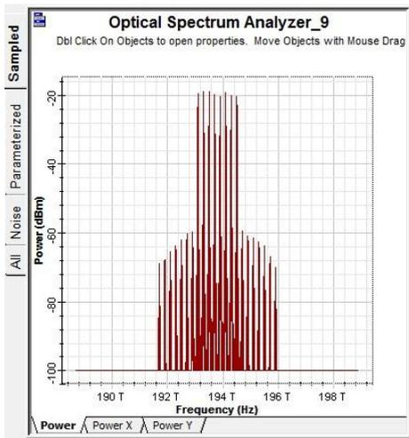
Figure 5: Output Spectrum for 8 Channels & 5 dbm Input Power
