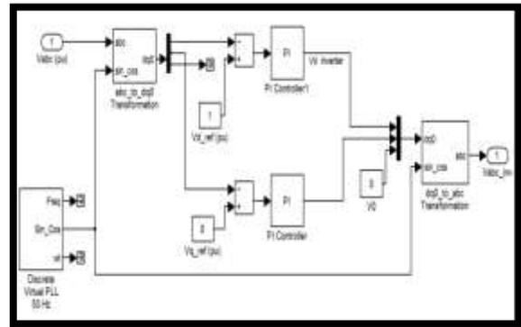
Figure 3.2: Constant Voltage Control Block Diagram
