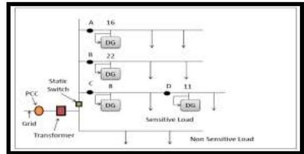
Fig.1 Basic Micro-grid Architecture
