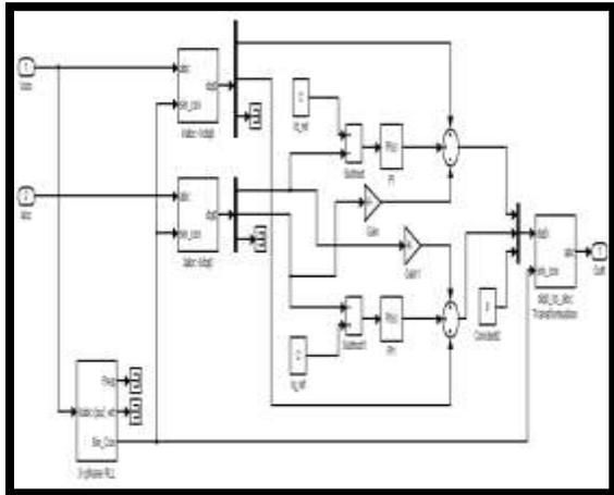
Figure 3.1: Current Control Block Diagram
