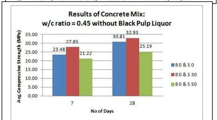
Fig. 4 B. Compressive Strength Results without Black Pulp Liquor..
