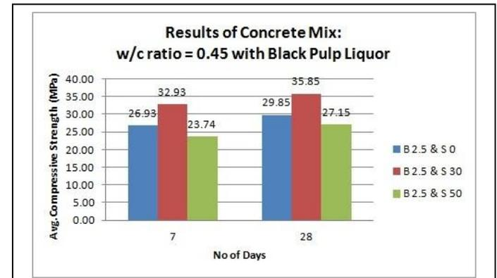
Fig. 4 A. Compressive Strength Results with Black Pulp Liquor.
