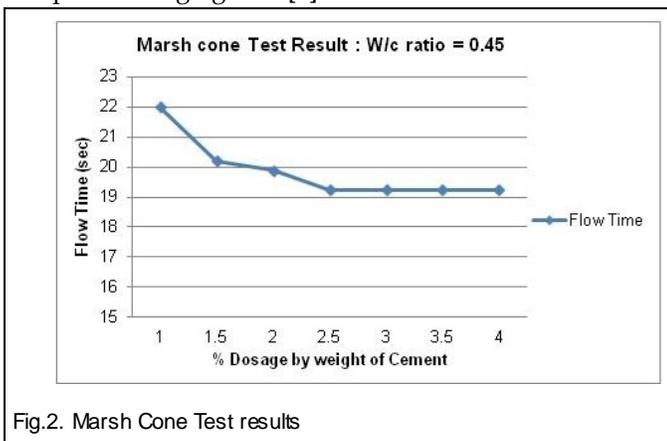
Fig.2. Marsh Cone Test results
