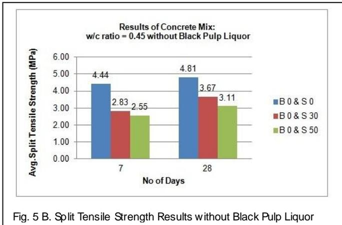
Fig. 5 B. Split Tensile Strength Results without Black Pulp Liquor
