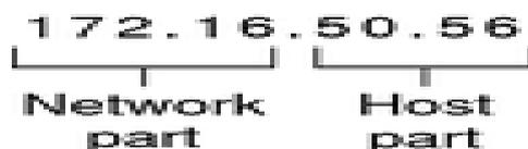
Figure 1. IPv4 Address Format [3]
