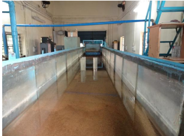
Fig. 3 Working section of a flume
