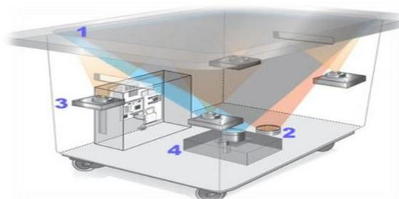
Figure 5. Hardware of a Surface Computer[10]
