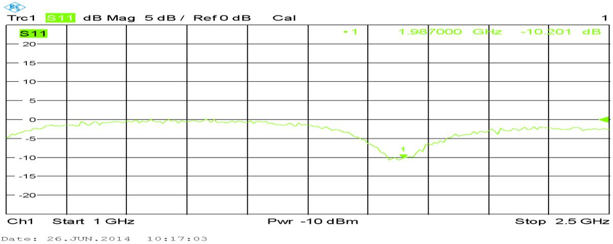
Fig 5.1: Frequency v/s Return loss
