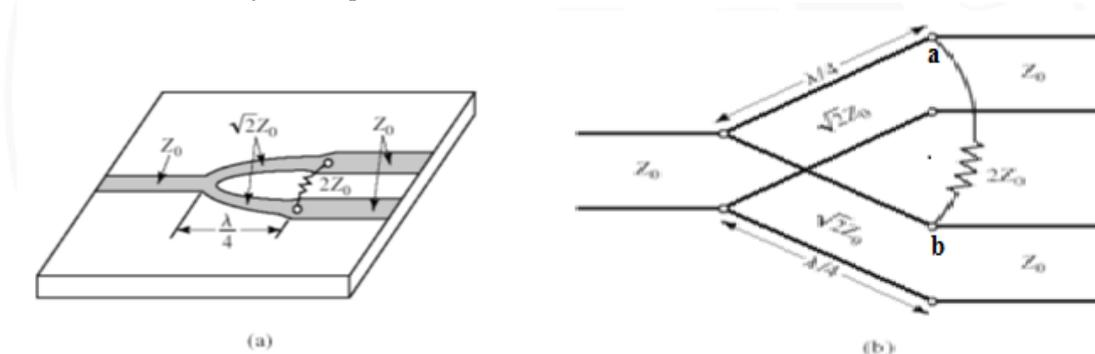
Fig. 1.1: The Wilkinson power divider. (a) An equal-split Wilkinson power divider in microstrip form. (b) Equivalent transmission line circuit
