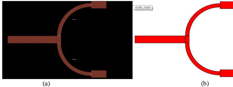
Fig: 3.1(a) Layout of the Wilkinson Power Divider, (b) Gerber file
