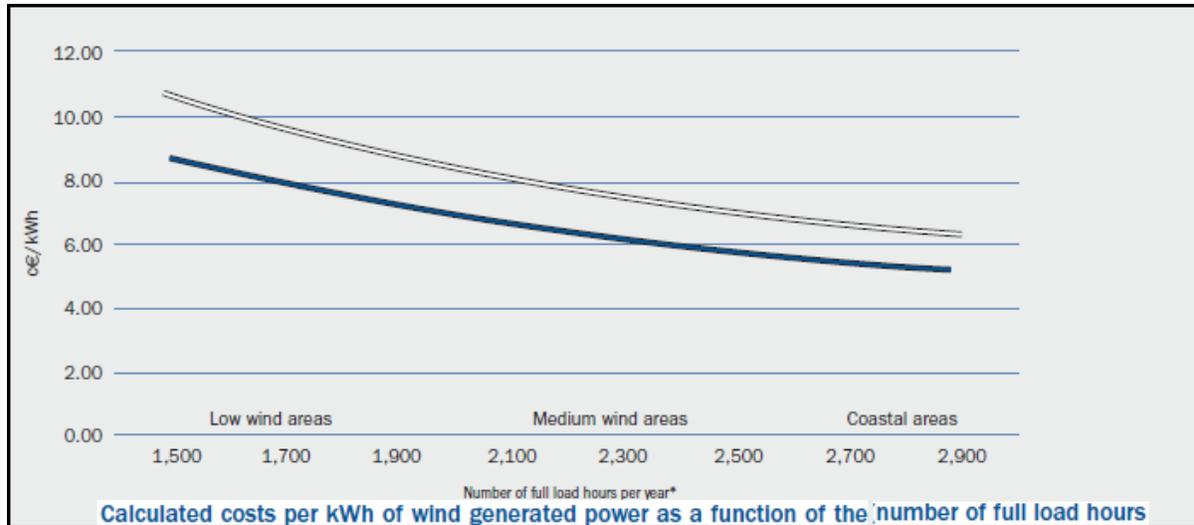
Figure 5: Cost of per kWh as a function of full load hours
