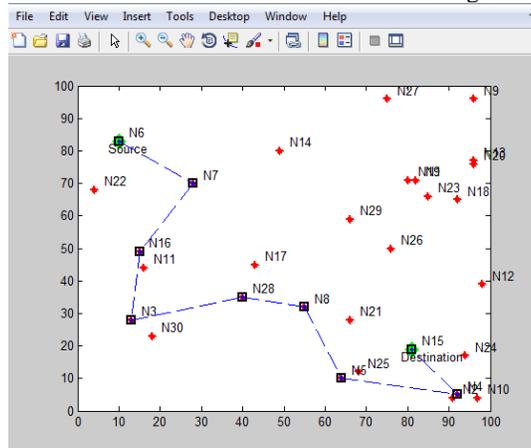
**Figure 1.5: Optimized path in a network**
