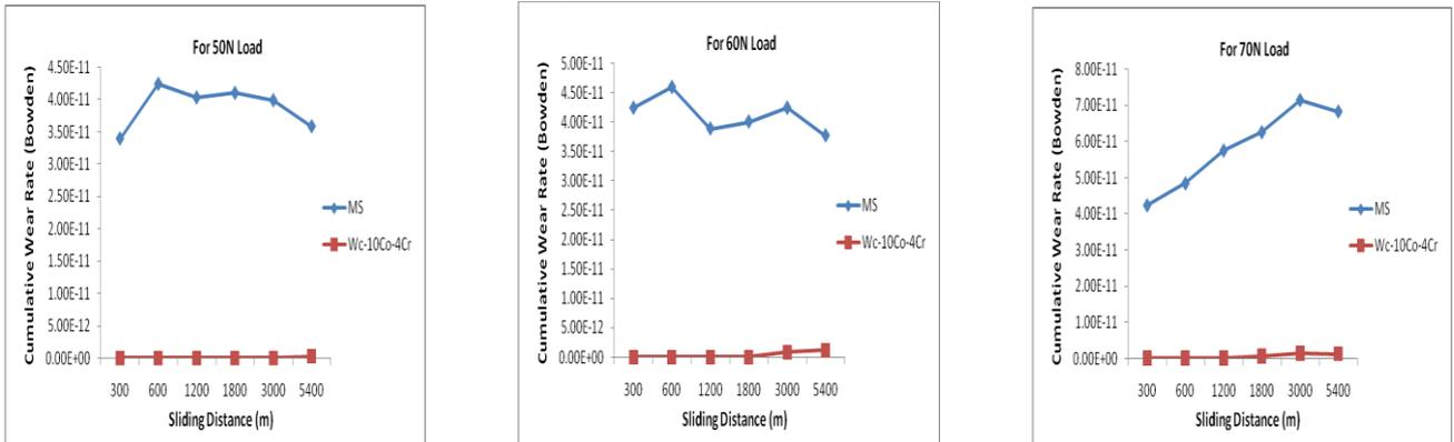
Fig. 4 cumulative wear rate for the uncoated, the detonation sprayed Wc-10Co-4Cr coated MS steel subjected to wear at normal loads of 50N, 60N and 70 N and sliding velocity of 1m/sec
