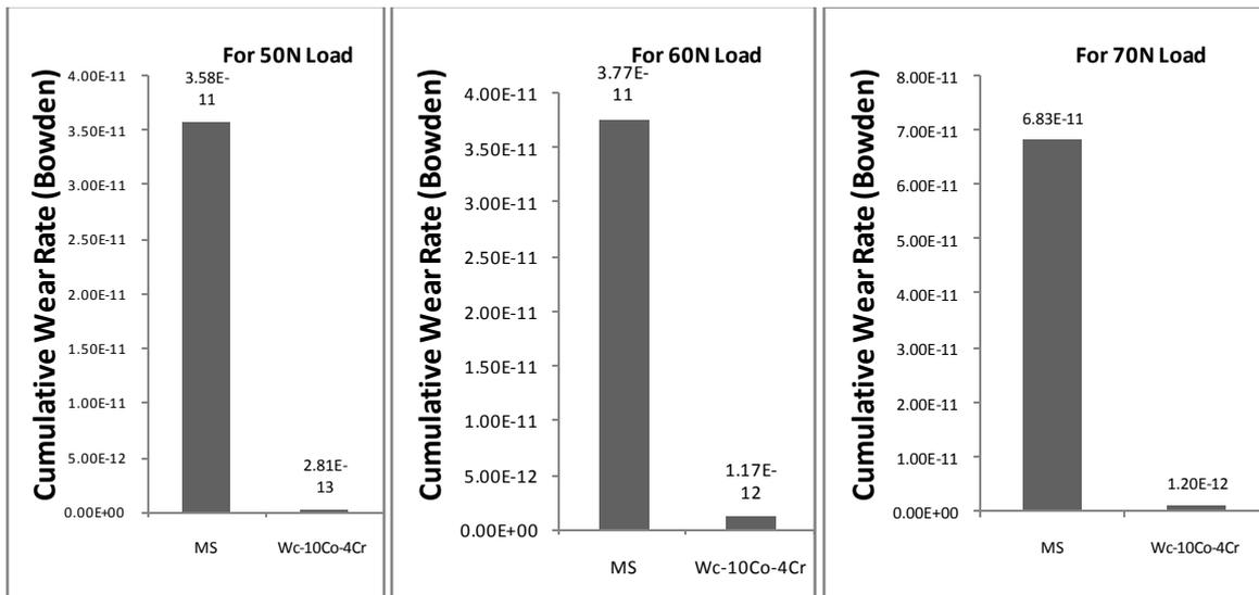
Fig. 5 Cumulative wear rate for the uncoated, the detonation sprayed Wc-10Co-4Cr coated MS steel subjected to wear at normal load of 70 N and sliding velocity of 1 m/sec after a sliding distance of 5400 meters.
