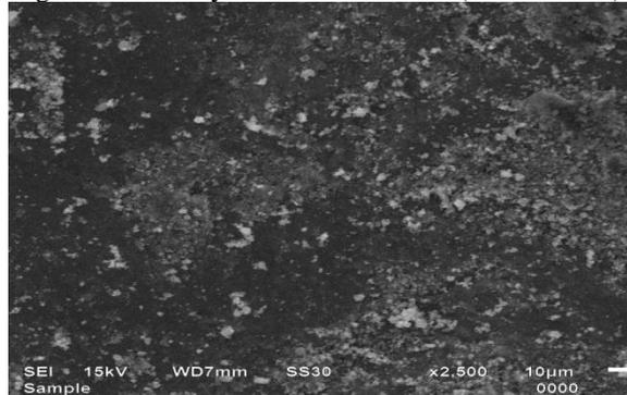
Fig.11 SEM analysis of detonation sprayed Wc-10Co-4Cr coated MS (At 70N load).
