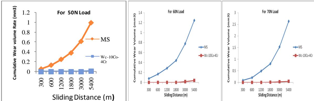
Fig. 6 cumulative wear volume for the uncoated, the detonation sprayed Wc-10Co-4Cr coated MS steel subjected to wear at normal loads of 50N, 60N and 70 N and sliding velocity of 1m/sec.
