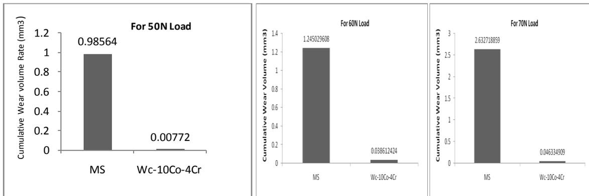
Fig. 7 Cumulative wear rate for the uncoated, the detonation sprayed Wc-10Co-4Cr coated MS steel subjected to wear at normal load of 50N, 60N and 70 N and sliding velocity of 1 m/sec after a sliding distance of 5400 meters.
