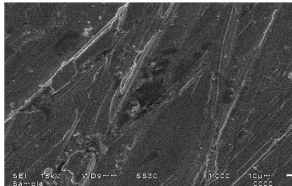
Fig.10 SEM analysis of uncoated MS (At 70N load).
