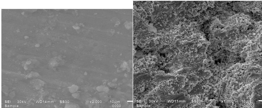
Fig. 8 SEM analysis of uncoated MS (without load).
