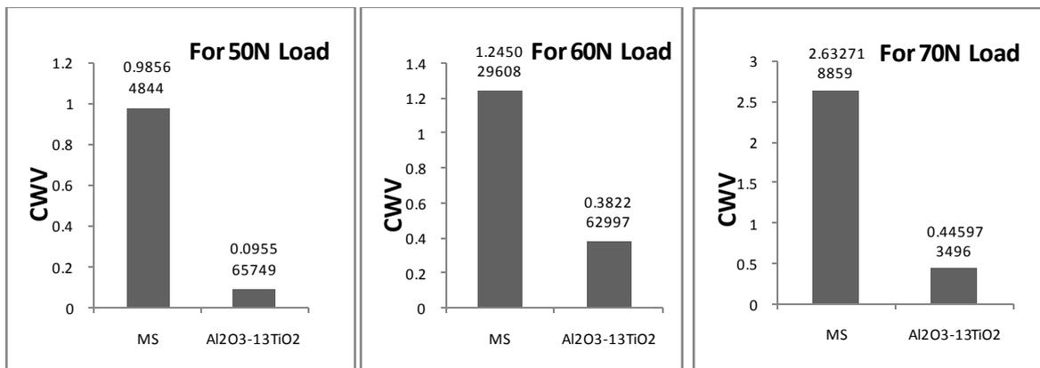
Fig. 7 Cumulative wear rate for the uncoated, the detonation sprayed Al<sub>2</sub>O<sub>3</sub>-13TiO<sub>2</sub> coated MS steel subjected to wear at normal load of 50N, 60N and 70 N and sliding velocity of 1 m/sec after a sliding distance of 5400 meters.
