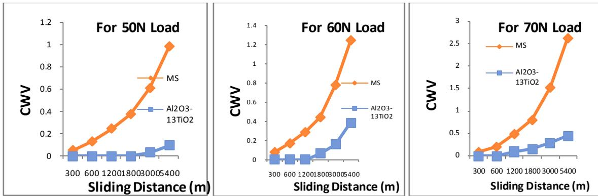
Fig. 5 cumulative wear volume for the uncoated, the detonation sprayed Al<sub>2</sub>O<sub>3</sub>-13TiO<sub>2</sub> coated MS steel subjected to wear at normal loads of 50N, 60N and 70 N and sliding velocity of 1m/sec.
