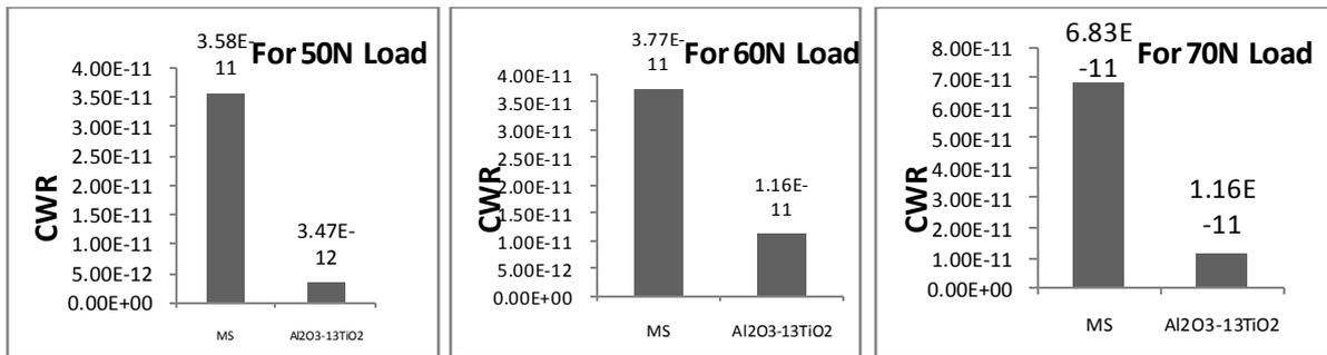
Fig. 5 Cumulative wear rate for the uncoated, the detonation sprayed  $\text{Al}_2\text{O}_3\text{-13TiO}_2$  coated MS steel subjected to wear at normal load of 70 N and sliding velocity of 1 m/sec after a sliding distance of 5400 meters.
