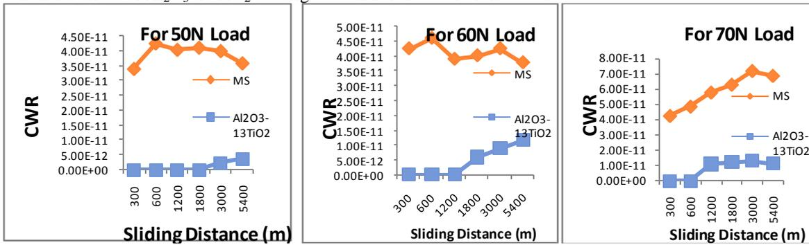
Fig. 4 cumulative wear rate for the uncoated, the detonation sprayed  $\text{Al}_2\text{O}_3\text{-13TiO}_2$  coated MS steel subjected to wear at normal loads of 50N, 60N and 70 N and sliding velocity of 1m/sec
