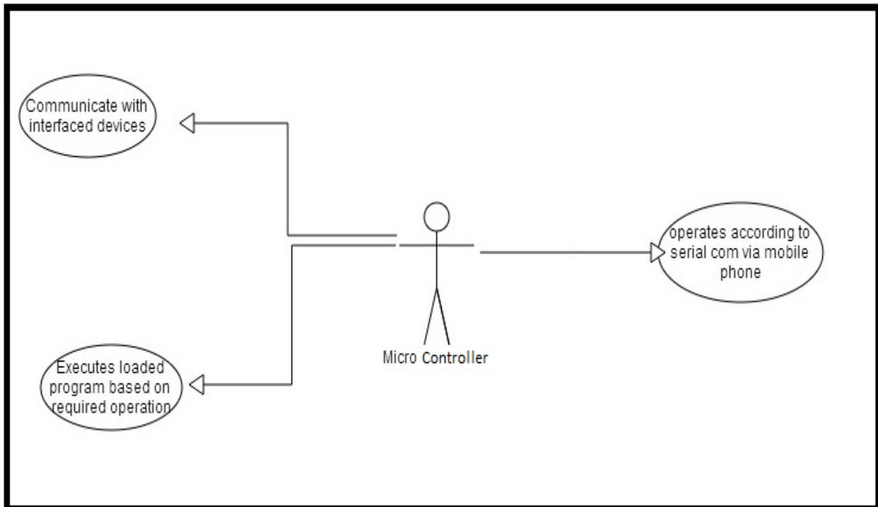
Fig 3 Use case for Microcontroller
