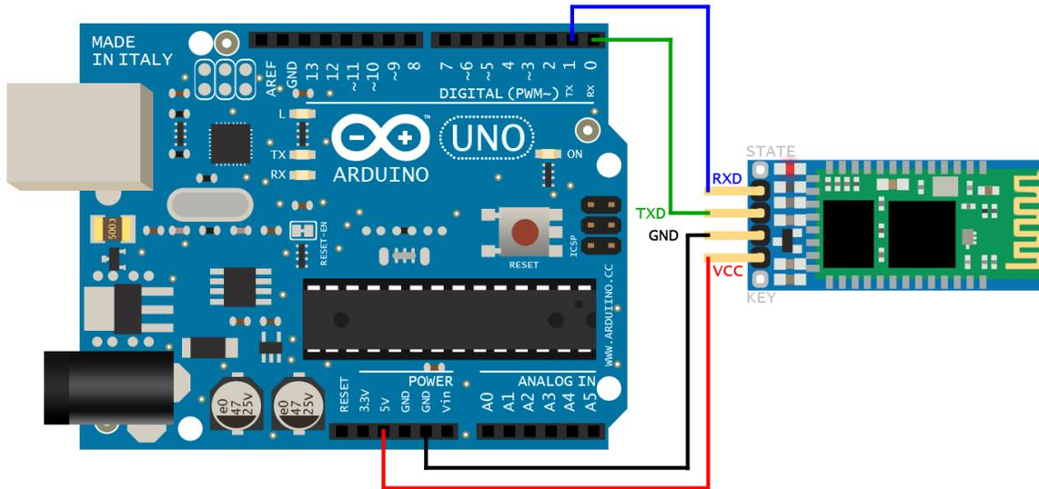
Fig 8 Bluetooth Shield Interfacing
