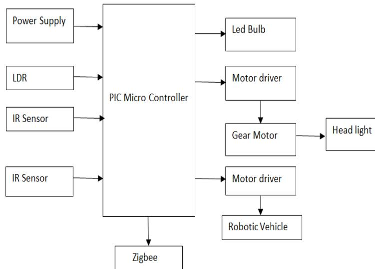
**Figure 1** Master block diagram
