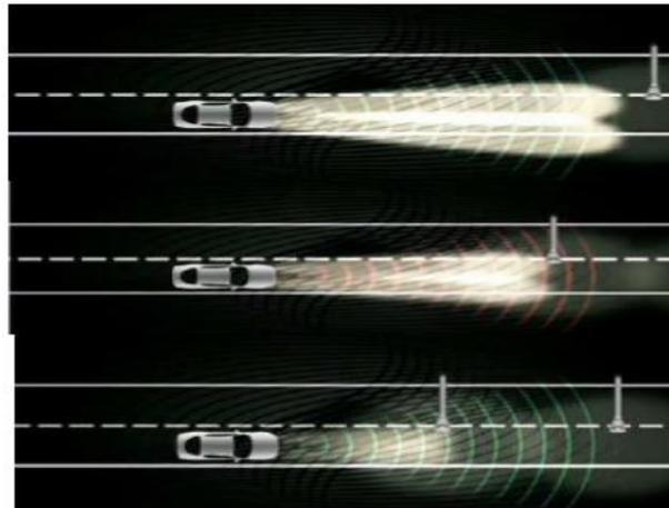
**Figure 3**Headlight intensity control system
