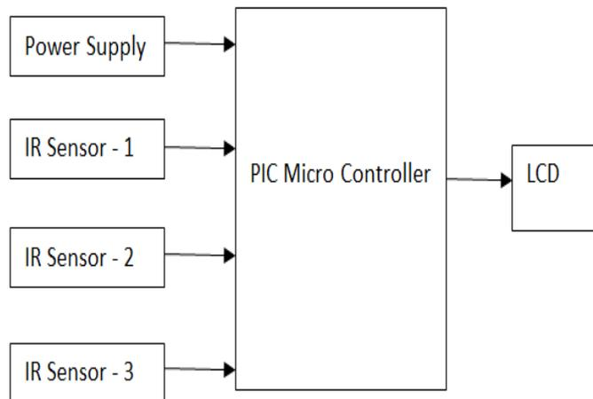
**Figure 2** Slave block diagram
