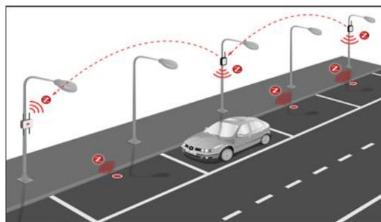
Figure 7 Smart parking system using IR sensor
