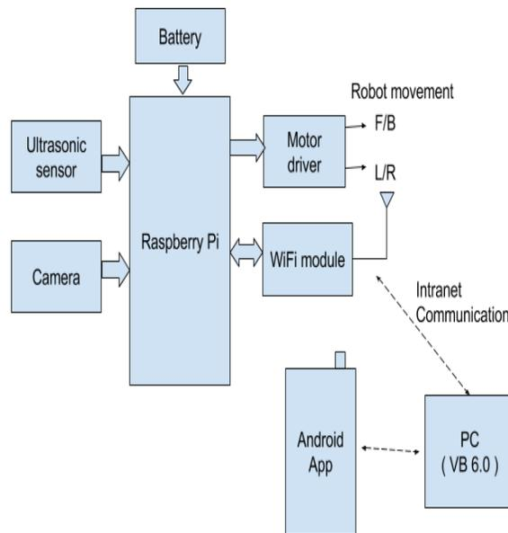
Fig2. Block Diagram
