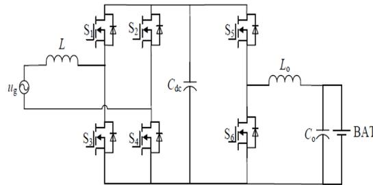
**Figure 1.** Topology of non-isolated on-board bidirectional charger composed of pulse width modulation (PWM) converter and bidirectional buck-boost DC-DC converter.
