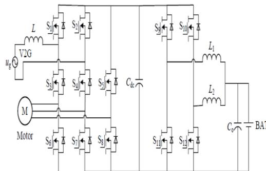
**Figure 3.** Topology of non-isolated integrated bidirectional charger composed of eight-switch inverter (ESI) and interleaved DC-DC converter.
