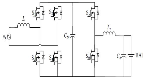
**Figure 2.** Topology of non-isolated on-board bidirectional charger composed of PWM converter and cascaded buck-boost DC-DC converter.
