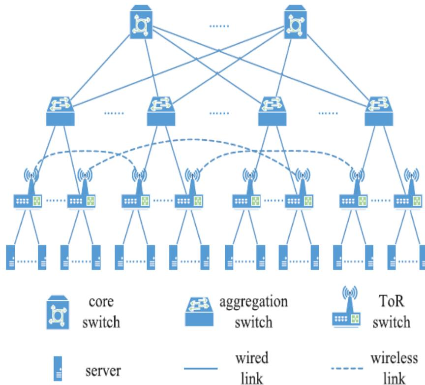
**Figure 1: Structure of a hybrid data center network. All ToR switches are equipped with a directional antenna on each to establish a wireless network among ToR switches in an on-demand manner.**
