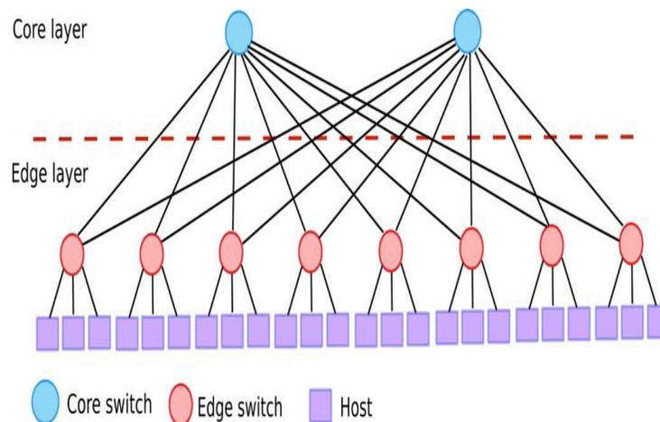
**Fig. 4. An example of a Two-Tier DCN with only core and edge layers. It consists of 10 switches, 24 hosts, and 40 links.**
