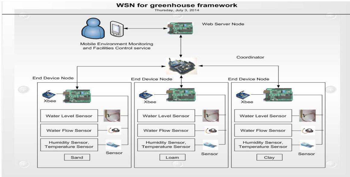
**Fig 3 Sensor data collection and irrigation control**
