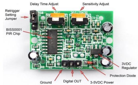
**Fig 8 Passive infrared sensor**
