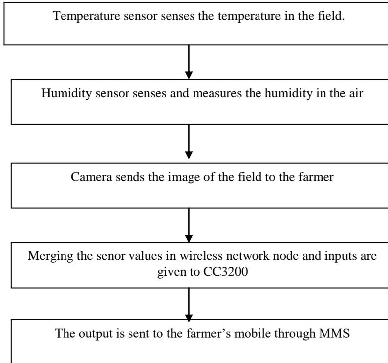
**Fig 1 Iot based monitoring system in smart agriculture**
