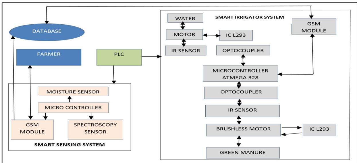
**Fig 2 Smart farming system using sensors**
