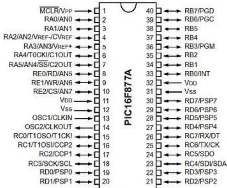
**Fig 6 PIC Microcontroller**
