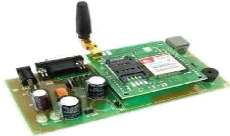
**Fig . 4 GSM module**
