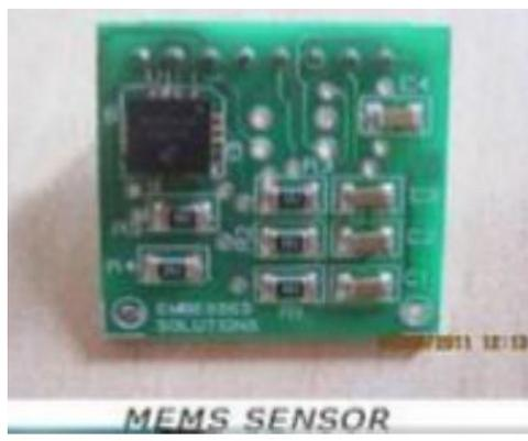
**Fig.7 MEMS Sensor**
