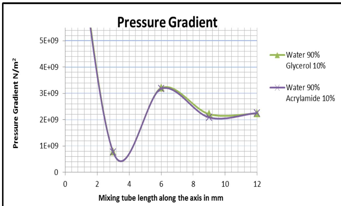
Fig 4.5(a) Pressure Gradient vs. Mixing Chamber
