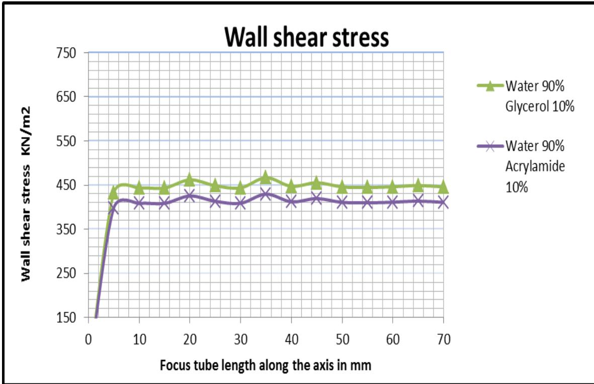
Fig 4.2[b] Wall shear stress vs. Focus tube
