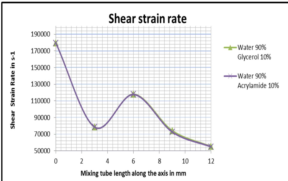
Fig 4.3(a) Shear Strain Rate vs. Mixing Chamber
