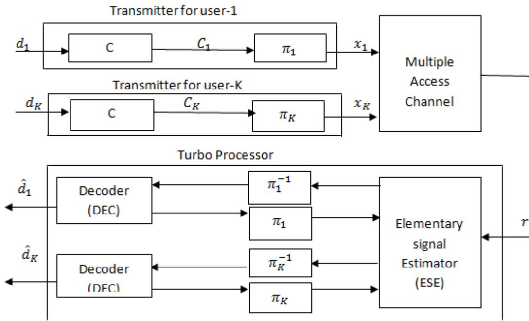
Fig.2 Transmitter and receiver structures of IDMA
