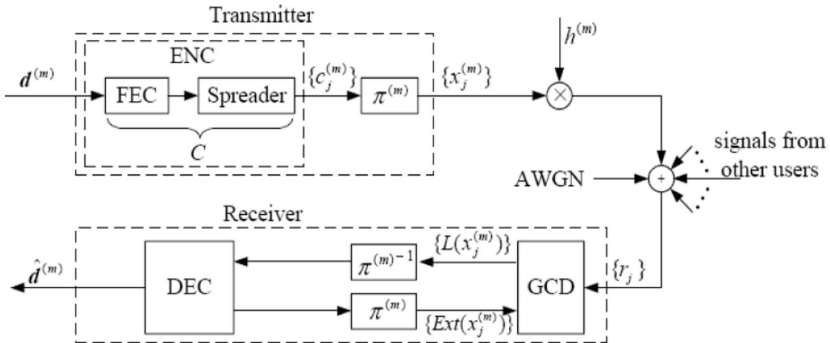
Fig.3 Transmitter and receiver structures of IDMA
