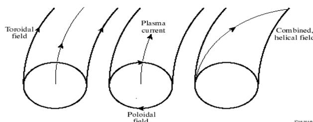
**Fig. 4. The tokamak's toroidal magnetic field combines with the poloidal field of the plasma current to produce a magnetic field with helical field lines.**
