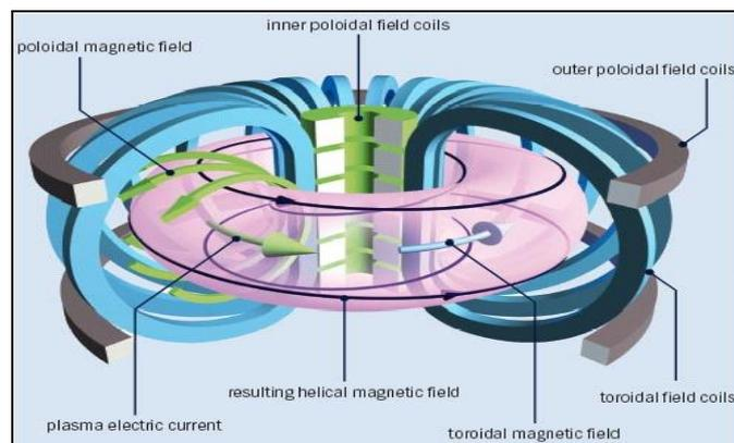
**Fig. 3. Magnetics field coils**
