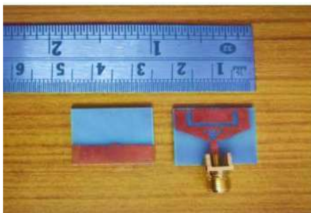
Figure 12 shows the practical design of UWB antenna connected with SMA connectors.
