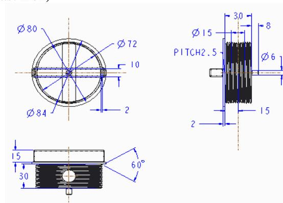
Figure 8. External threaded nut
