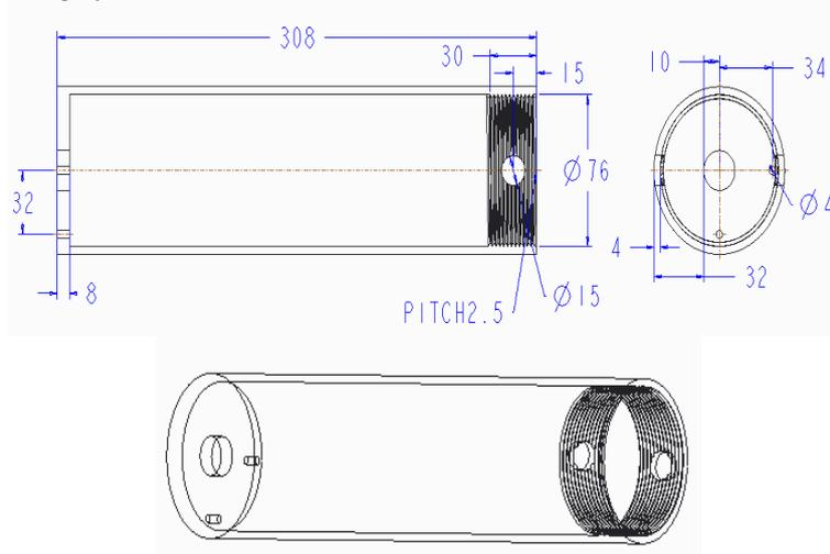
Figure 7. Casing cylinder
