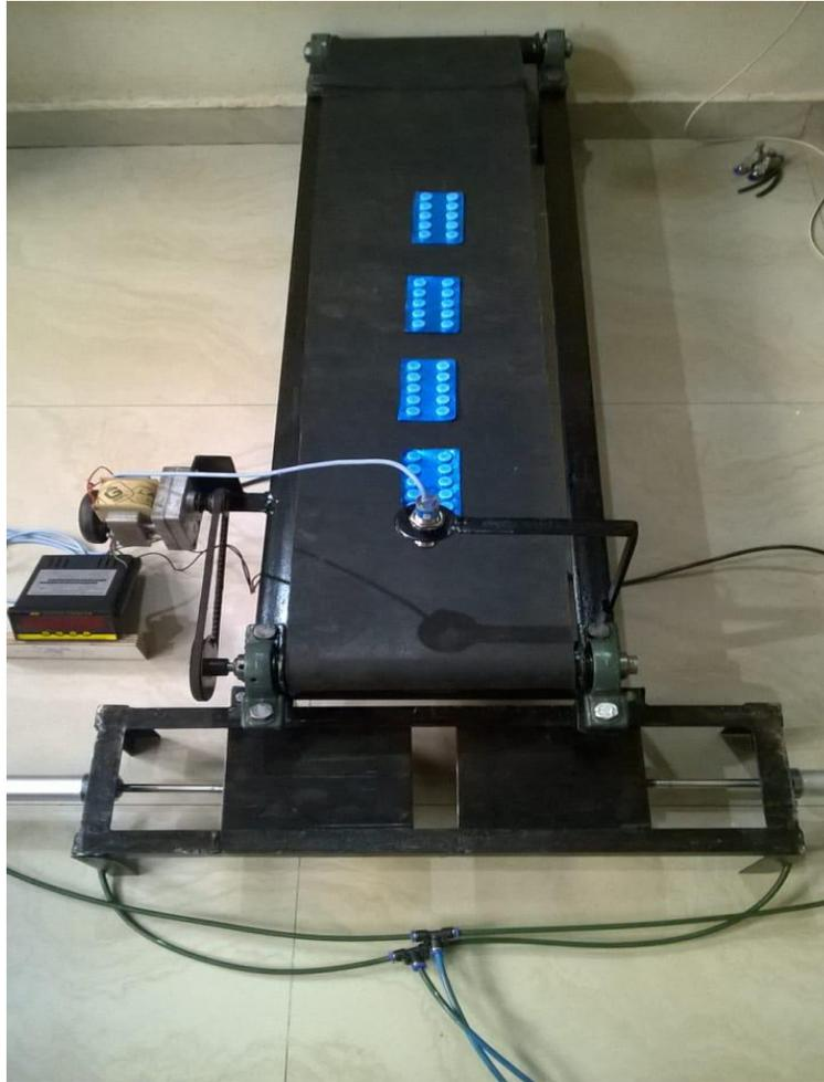
**Figure 1. Propose automatic tablet counting & shifting mechanism in belt conveyor**
