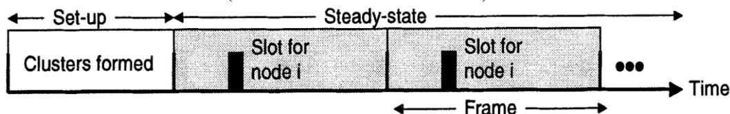
**Figure 2 Time line showing LEACH operation.**
