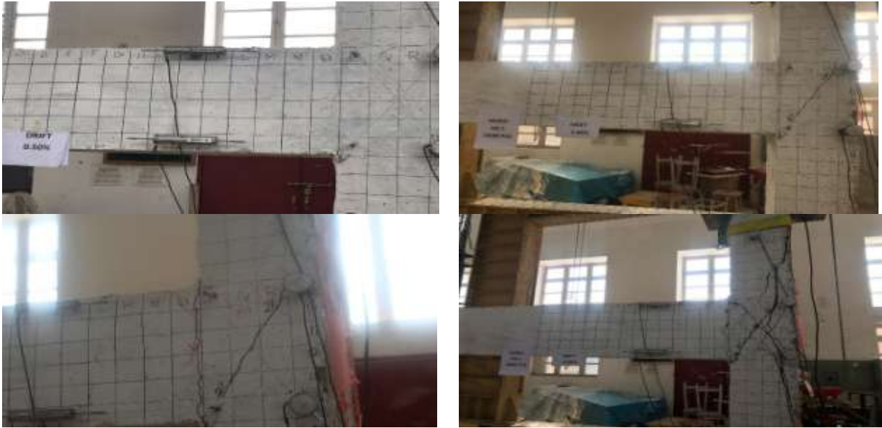
Figure 5: Damage pattern of tested models
