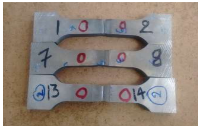
Fig. 6. Fractured specimens of weld joints formed from conical tip tool
