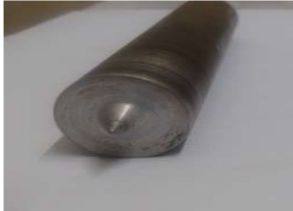
Fig. 3. Conical tip tool during experimentation
