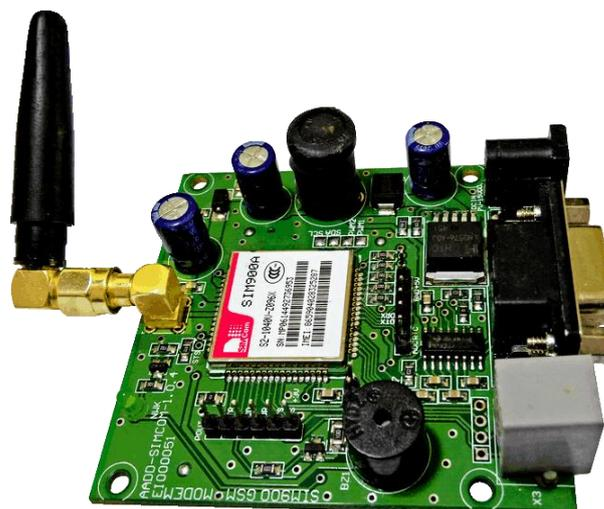
Figure1.1c: GSM module
