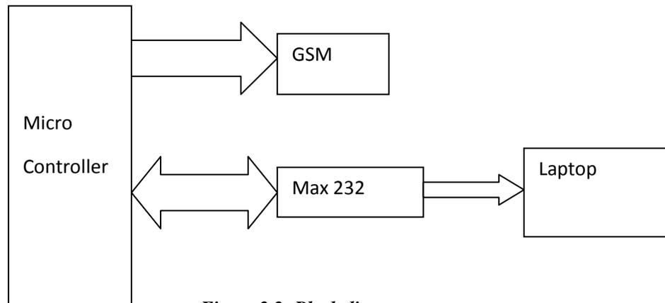
**Figure 2.2: Block diagram**
