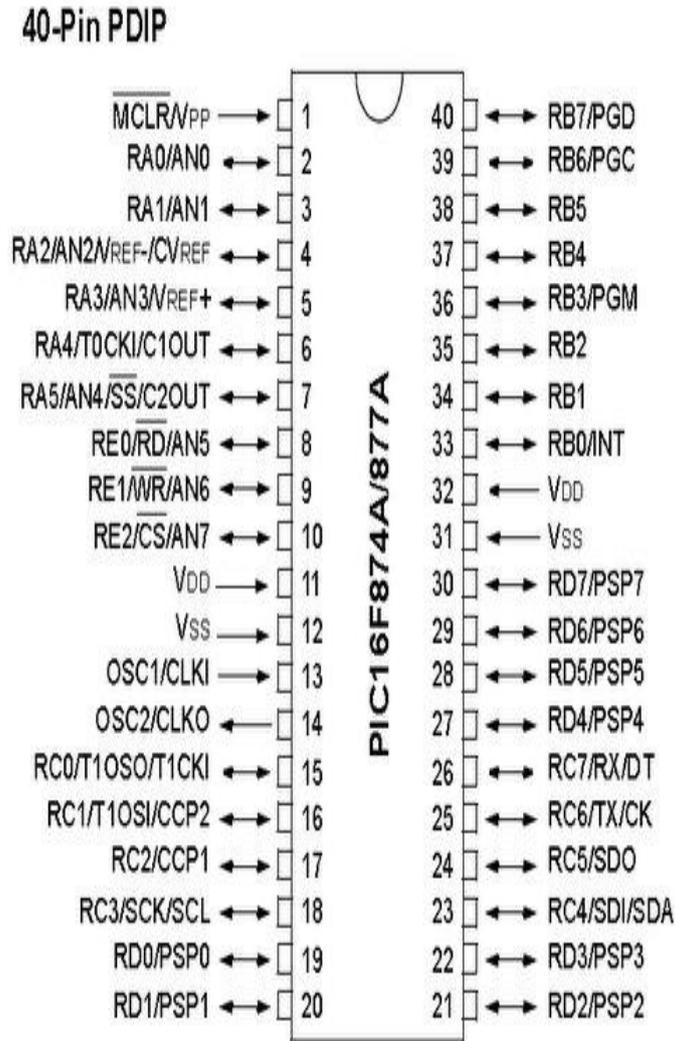
Figure1.1b: Pin diagram
