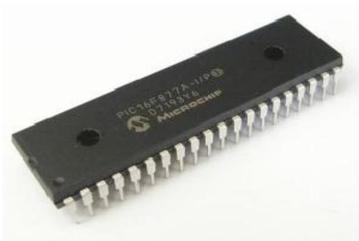
**Figure1.1a: PIC microcontroller**
