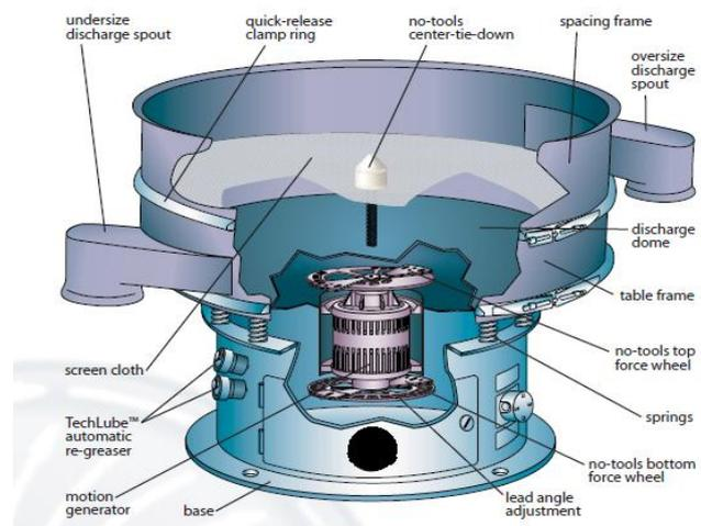
Fig 1.1 Vibratory Screening Machine
