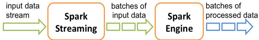
*Figure 4. Working of Spark Streaming*
