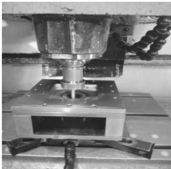
Fig 1.Incremental sheet metal forming process [5]
