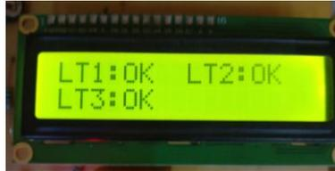
**Fig 3:Conditions of the street lights which is displayed on LCD screen**
