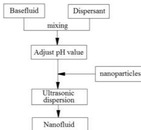
**Figure 02:** Two step preparation process of nanofluid.
