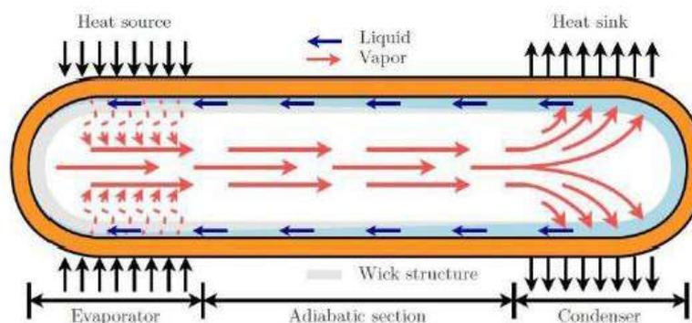
Figure 01. Heat pipe. <sup>[16]</sup>
