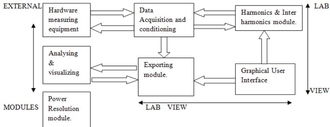
*Fig: 2 Power Monitoring system*
