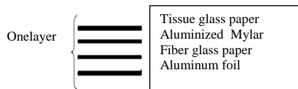
Whole blanket of composite material is wrapped on the test and guard chambers of calorimeter with layer density is 10 layers/cm. with insulation thickness is 20 mm. The specification of our samples is shown in table-2.
