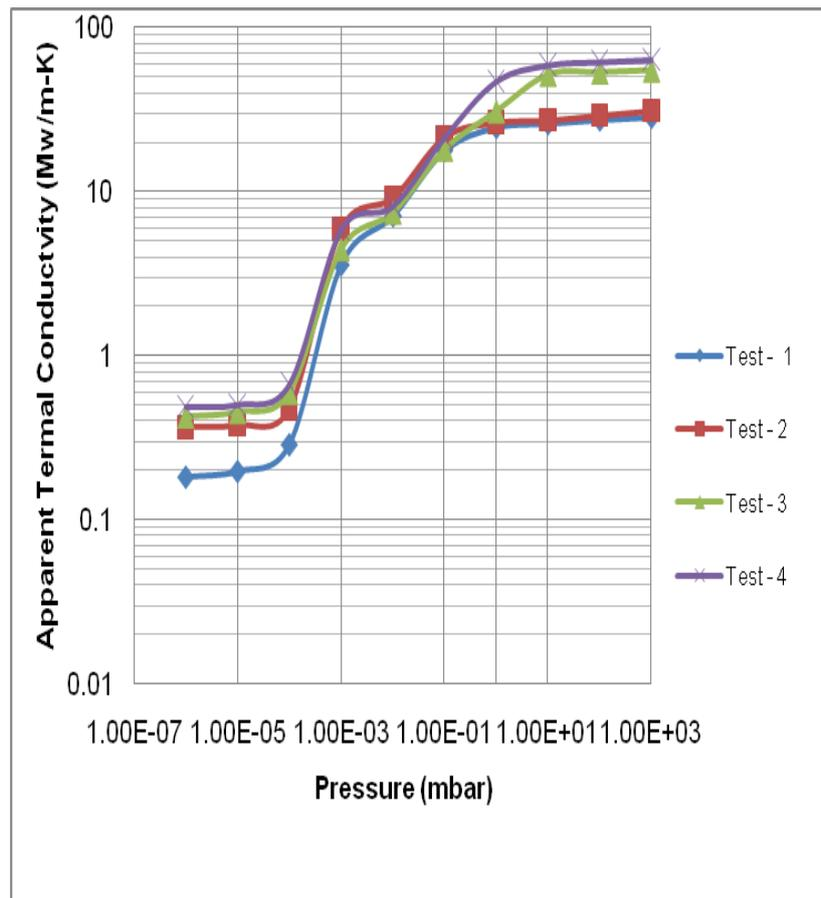
**Figure 3. Variation of apparent thermal Conductivity with vacuum chamber pressure.**
