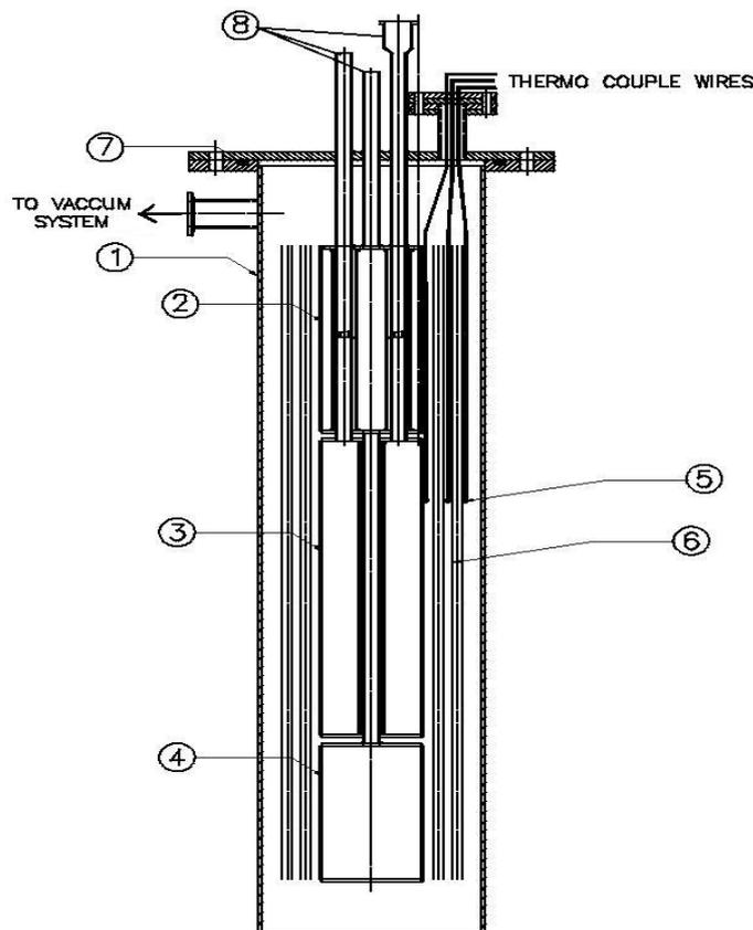
**Figure 2 Calorimeter for Measurement of Apparent Mean Thermal Conductivity of MLI**
