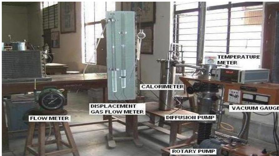
**Figure 1 Overall views of experimental set-up**
