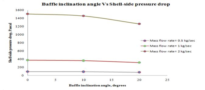
Fig.4 Variation of pressure drop with baffle inclination angle (for 0.5 kg/s, 1 kg/s, 2 kg/s mass flow rates)
