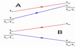
Fig 2. Counter current (A) and parallel (B) flows
