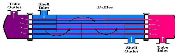
Fig 1. A Shell and Tube heat exchanger
