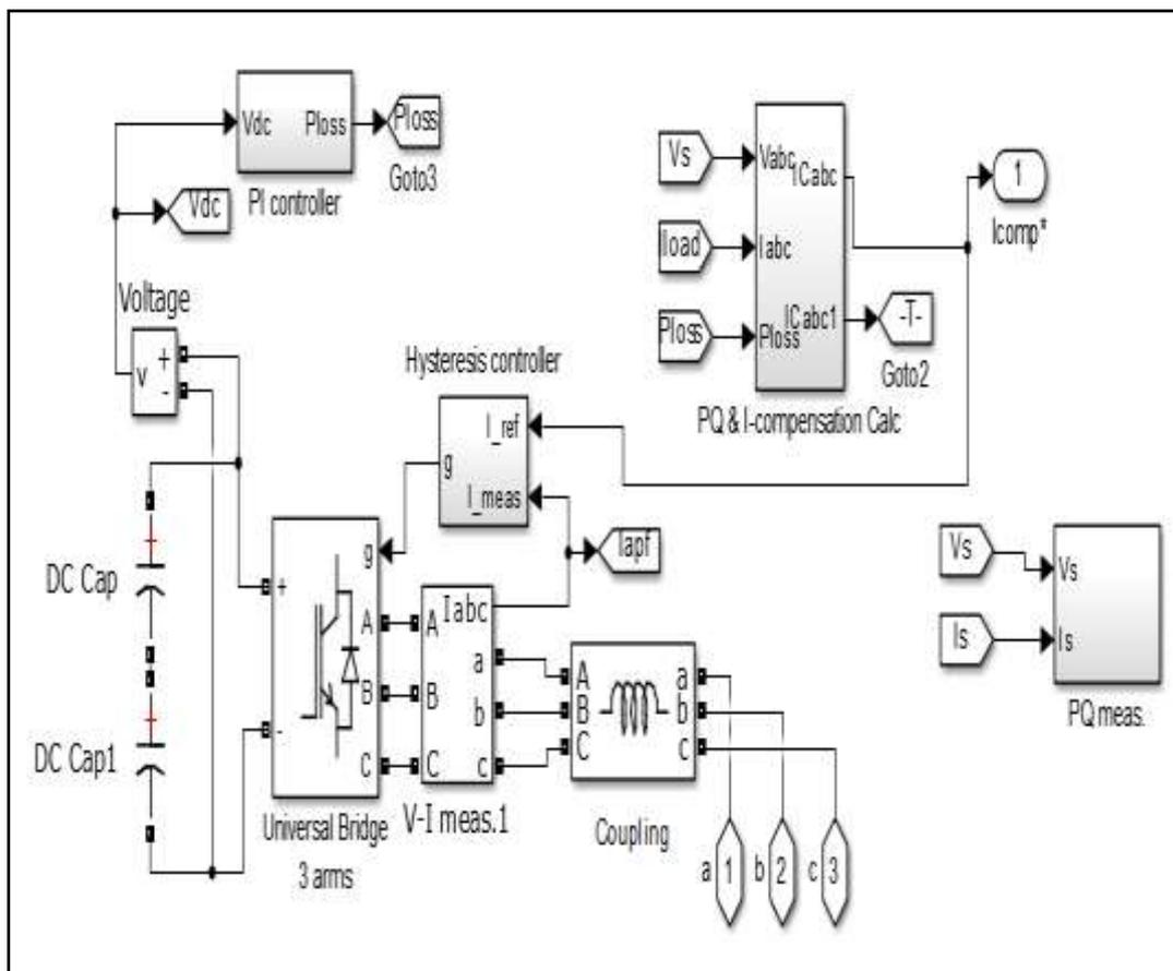
Figure8. STATCOM (shunt active power filter)
