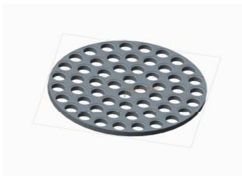
**Fig.2 Fifty five Cavity Bakelite Fixture for Rubber bushes**
