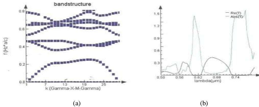
Fig 1 (a) Dispersion diagram of a perfect 2D photonic crystal calculated using the FDTD method. Silicon rods ( $n=12.083$ ) are defined in air in a square lattice where the radius of the holes is  $r=0.24a$ . (b) Transmission through the same photonic crystal in the  $\Gamma$ - $k$  direction obtained by FDTD method
