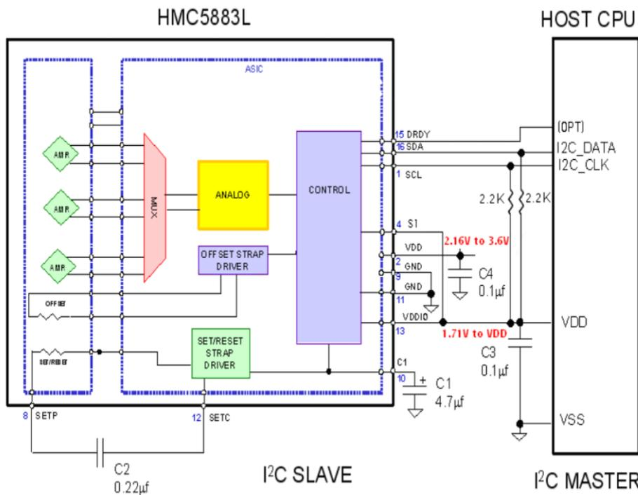
Fig 2: INTERNAL SCHEMATIC DIAGRAM
