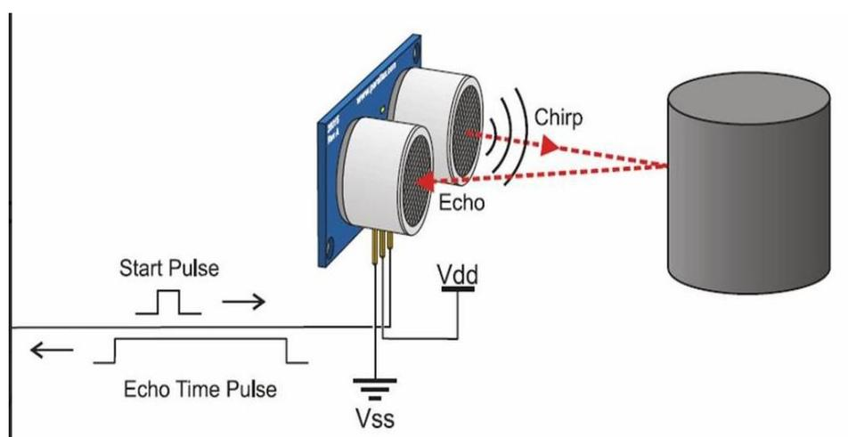
Fig. 3: Obstacle Detection Sensor Configuration
