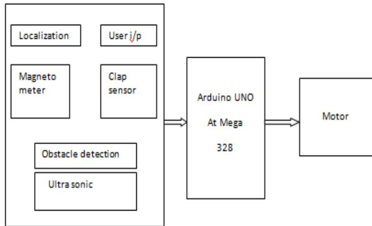
Fig 1: Embedded System with Input and Output Modules
