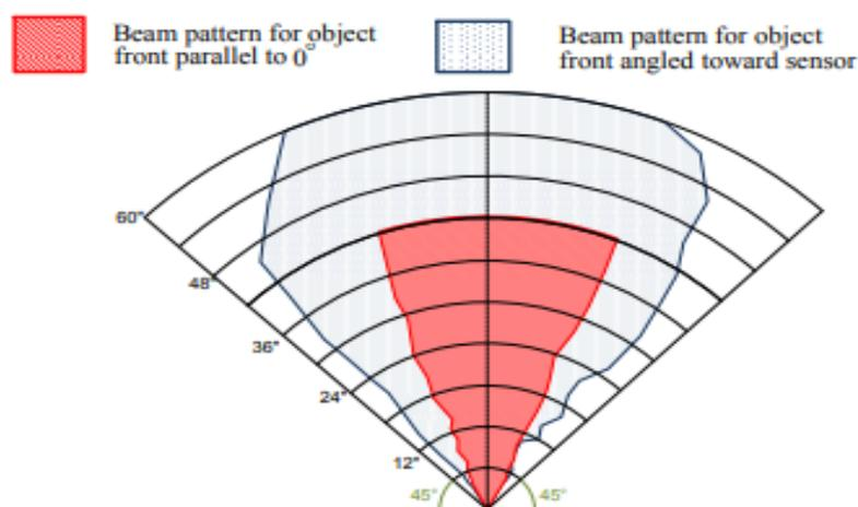
Fig. 4: Ultrasonic Sensor Beam Pattern
