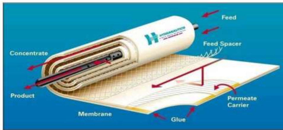
Figure 4: Process of Treatment Inside
