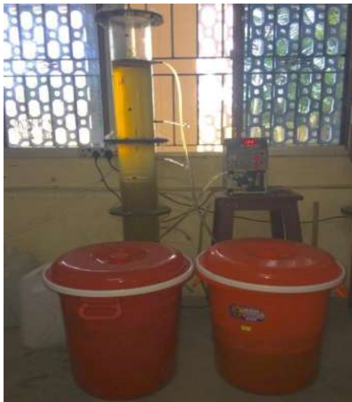
Fig. 3 Prototype UASBR model
