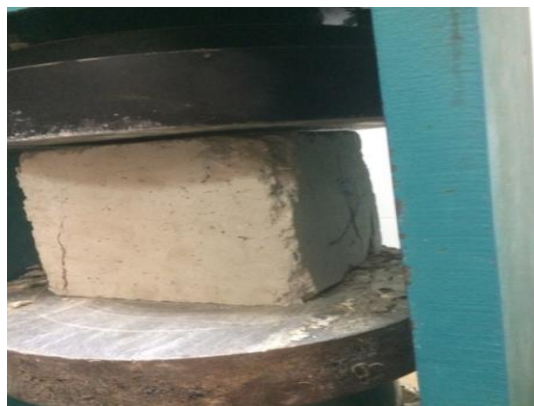
Fig. (5) Failure of cube D
