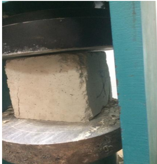
a) Fig. (2) First cracks
