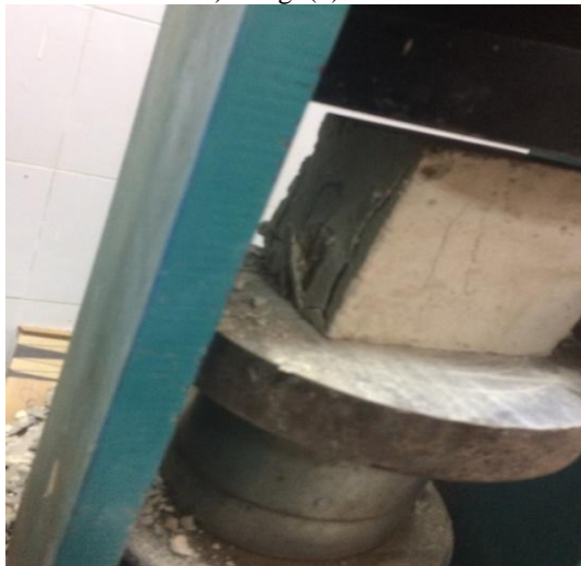
b) Fig. (2) Failure cracks
