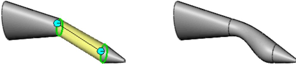
Fig.7 Seamless joint
