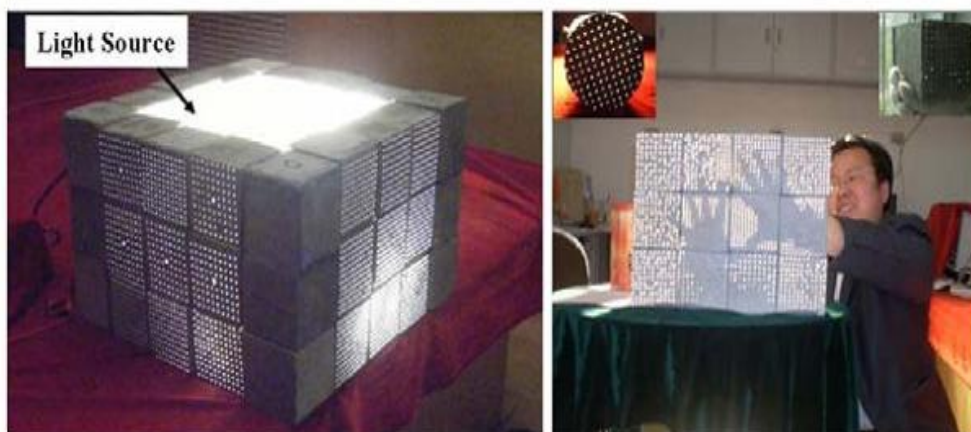
Figure:2 - Transparent demonstration of smart transparent concrete
