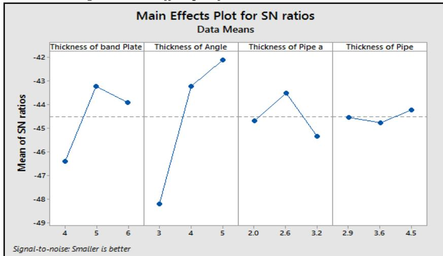
Figure 6 Main effect plot for S/N ratio data – shear stress
