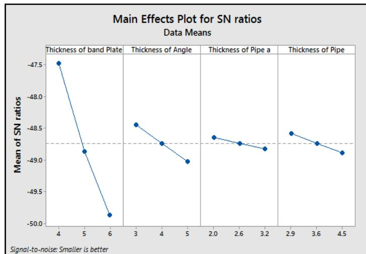
Figure 4: Main effect plot for S/N ratio data – weight
