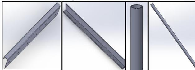
Figure 2: Band Plate, L-angle, Big pipe weldment, Small pipe weldment
