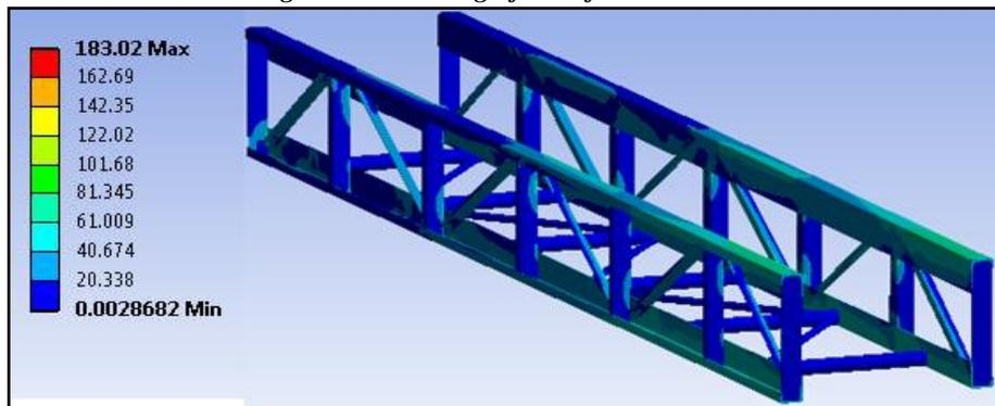
Figure 10: Shear stress in modified section
