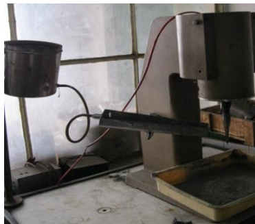
Fig.2 Ultrasonic drilling Machine set-up
