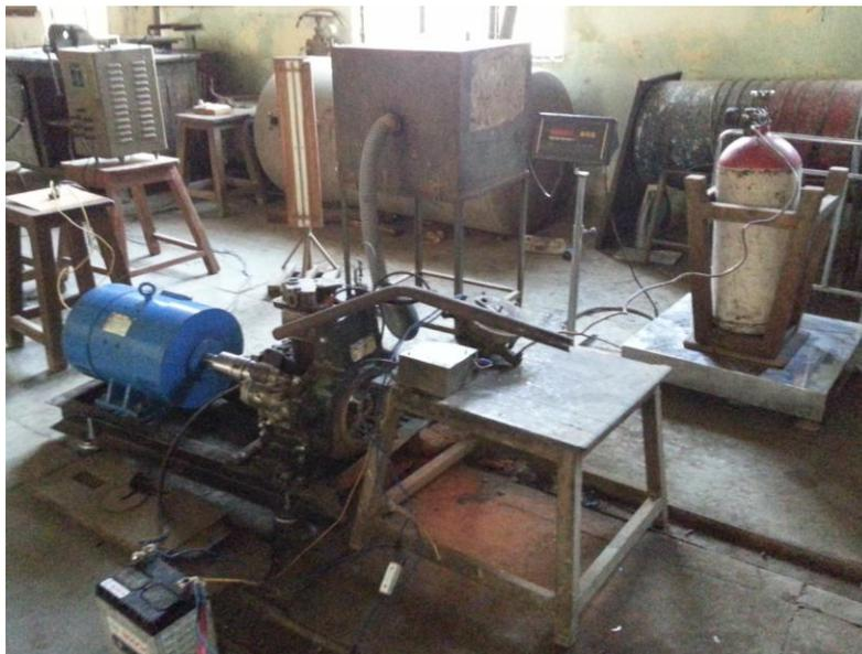
*Fig1. Actual experimental set-ups for modified engine (CNG engine)*
