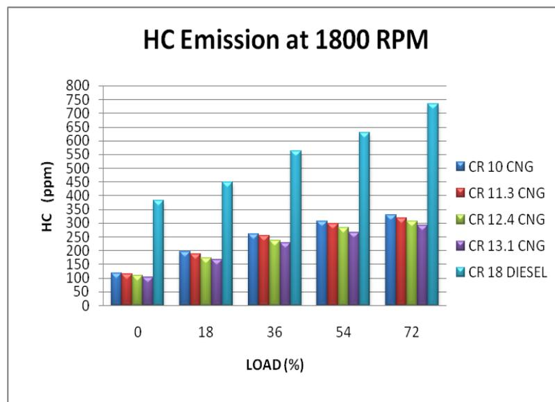
**Fig8. HC emission at 1800 rpm for both diesel and CNG at varying CR.**
