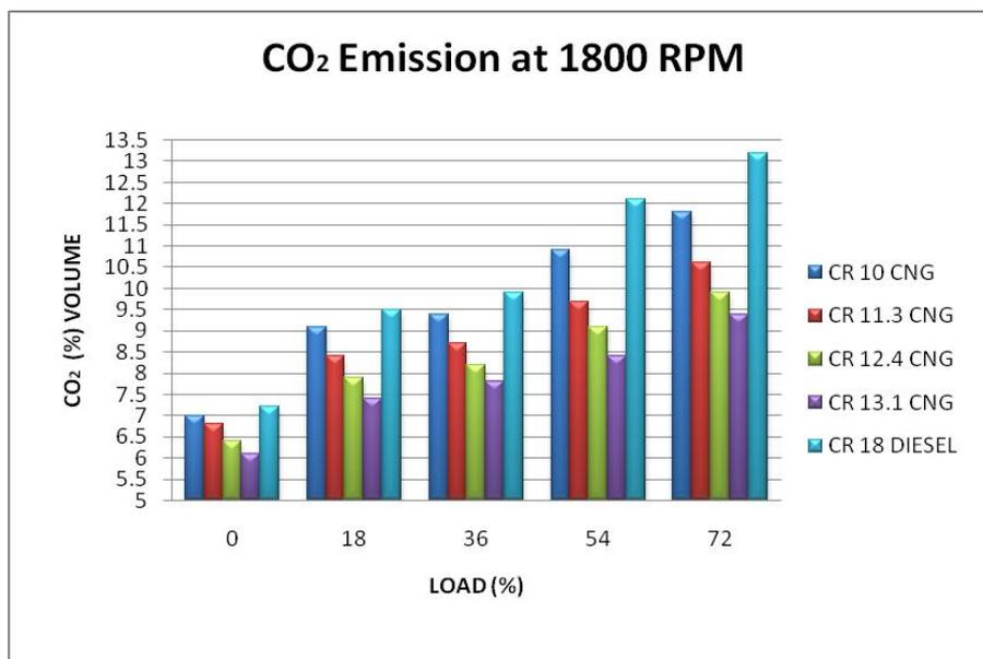
Fig6. CO<sub>2</sub> emission at 1800 rpm for both diesel and CNG at varying CR.
