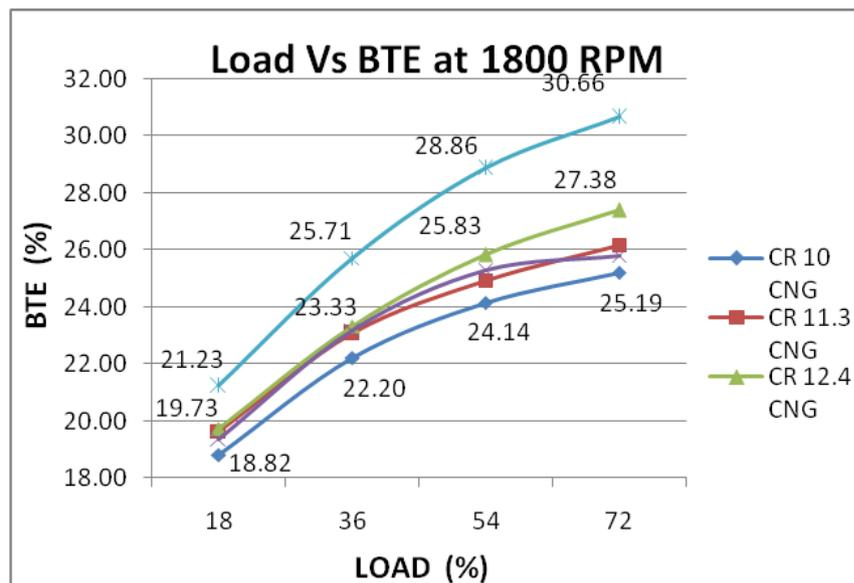
**Fig4. Load Vs Brake Thermal Efficiency at 1800 rpm for both diesel and CNG at varying CR.**
