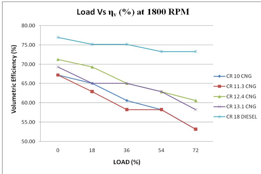
**Fig5. Load Vs Volumetric Efficiency at 1800 rpm for both diesel and CNG at varying CR.**
