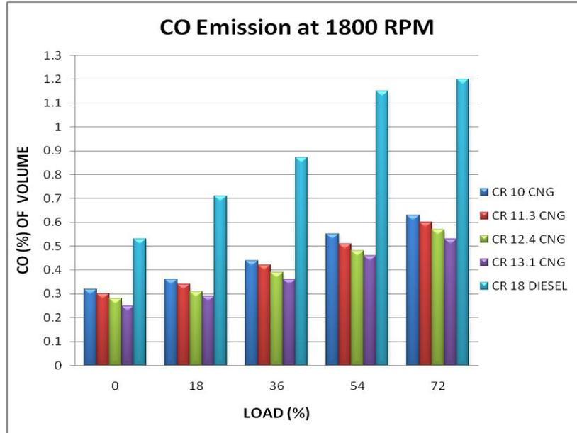
Fig7. CO emission at 1800 rpm for both diesel and CNG at varying CR.
