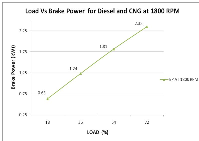
**Fig2. Load Vs Brake Power at 1800 rpm for both diesel and CNG.**
