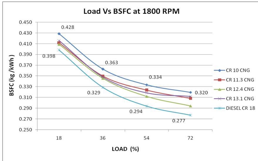
Fig3. Load Vs Brake Specific Fuel Consumption at 1800 rpm for both diesel and CNG at varying CR.
