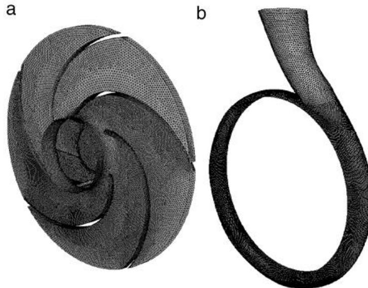
Figure 2.4. Impeller fluid region (a) and volute surface mesh (b) [11]
