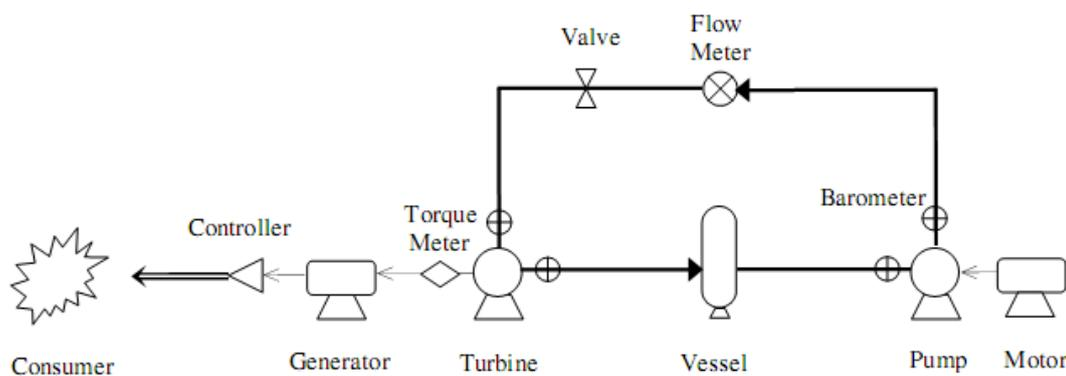
*Figure 2.3. The mini hydropower established in the University of Tehran [5]*
