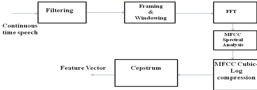
Fig.5.3. Block diagram for steps involving feature extraction.
