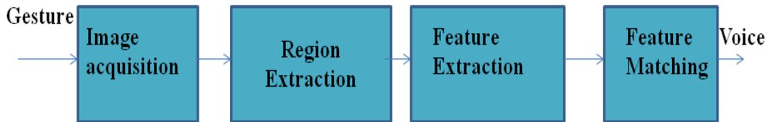
Fig .4.1 Block diagram of Gesture to sound conversion
